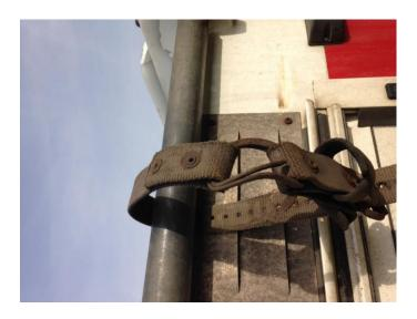
A UK based DNO has recently reported a significant near miss incident when a set of extending ladders fell from an overhead lines vehicle as it was travelling at speed along a major motorway. The potential consequences of any equipment falling from vehicles, regardless of the speed at which they are travelling, is extremely serious. The investigation found that only one securing strap had been used, and it is believed that this failed.
