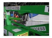
The initial investigation has identified that the weld connecting the head of the ram to the main body of the ram has failed. The cause of this is currently being further investigated, however, neither witness statements or CCTV footage of the incident indicate that the MEWP was struck immediately prior to the incident or during its time on site.
