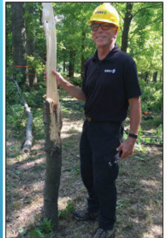
Image 5: Ward Peterson of Davey holds up a 6-inch pin oak branch torn off in a pull test. The stub was left alone to respond on its own, so the results of this “natural fracturing” can be studied. The break stopped near a node, which had no laterals but a lot of strength.
