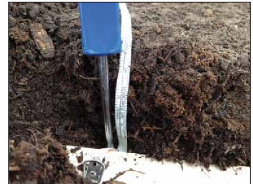
Section 83.3.5 states, "Mulch, soil, and other materials should be removed as needed to allow for inspection." After fresh mulch was removed, a 2" layer of compacted mulch remained above the soil. No root growth was found in this shredded hardwood, which looked and smelled as sterile as peat.
