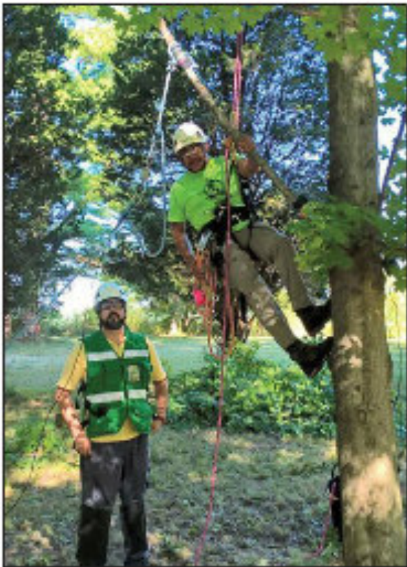
Image 4: By winching branches in two directions simultaneously, Adolfo Sanchez and Eduardo Medina were able to document the effects of combined static and torsional loading.
